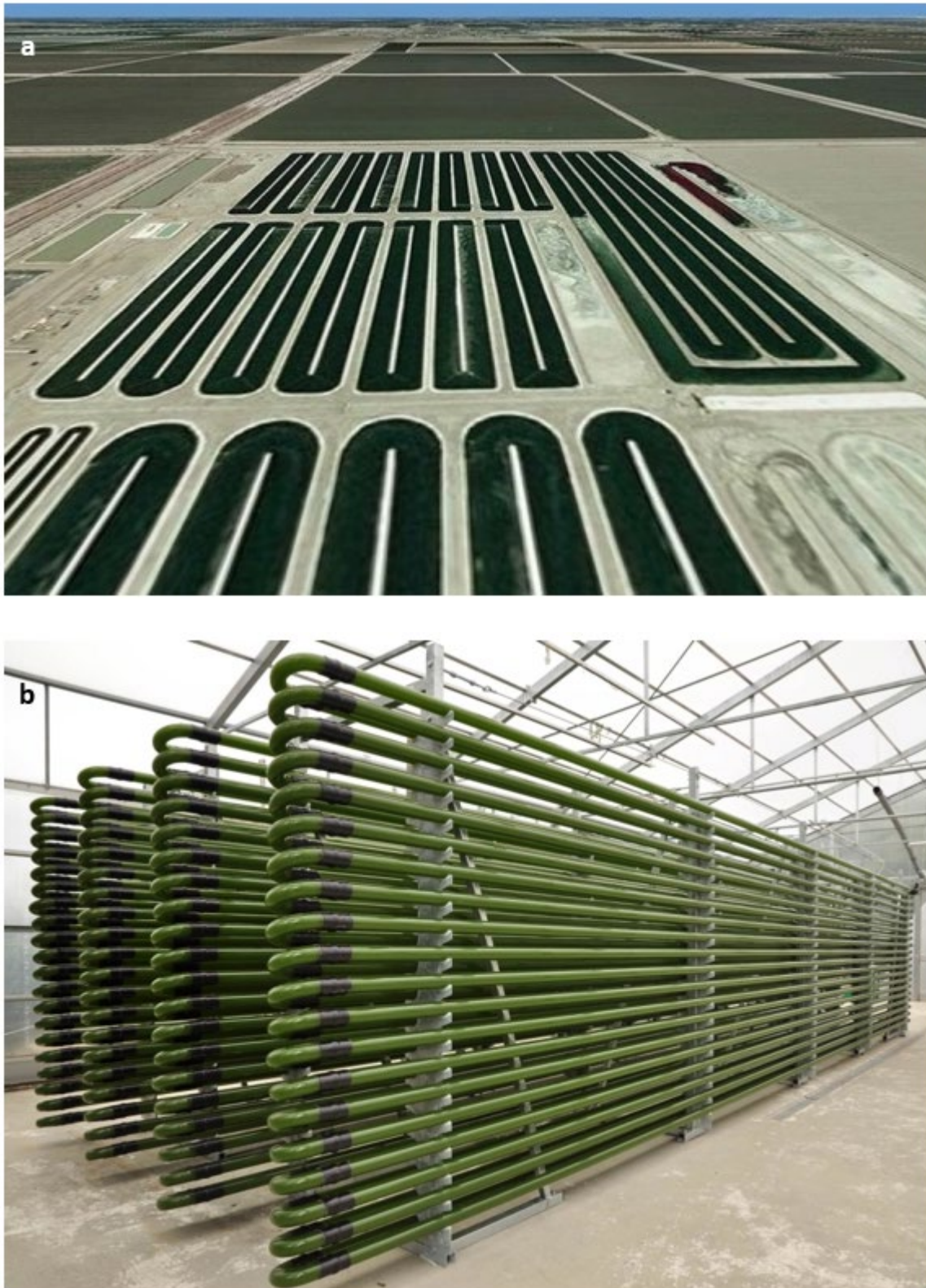
Figure 3 Production of microalgae in a) open raceway ponds, and b) a closed photo bioreactor. Image credits: Courtesy of US DOE/Pacific Northwest National Laboratory (via Flickr ); IGV Biotech (via Wikipedia ).
