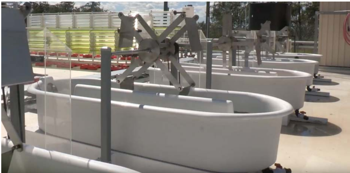
Figure 2 Small raceway ponds that would be used as culture vessels. These would be covered with secure lids during cultivation of the GMOs. Image supplied by applicant.
